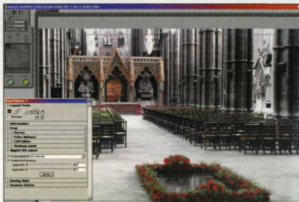
Above is an old faded slide with color shift toward red. Embedded ROC technology in the Nikon scanner corrects color, GEM reduces grain, and ICE removes scratches.
